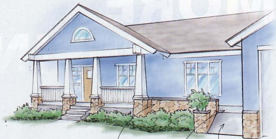
Stone veneer integrates with porch detail.
